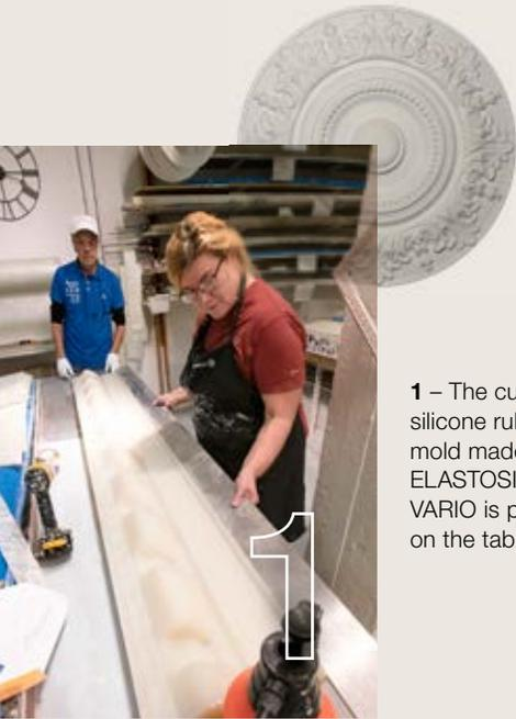
1 – The cured silicone rubber mold made from ELASTOSIL® VARIO is placed on the table.
