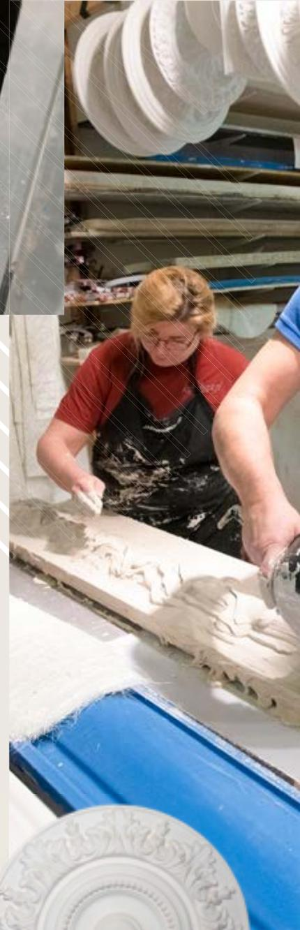
3 – A first layer of plaster is applied by brush to make sure no air bubbles form on the surface of the finished object later in the process.
